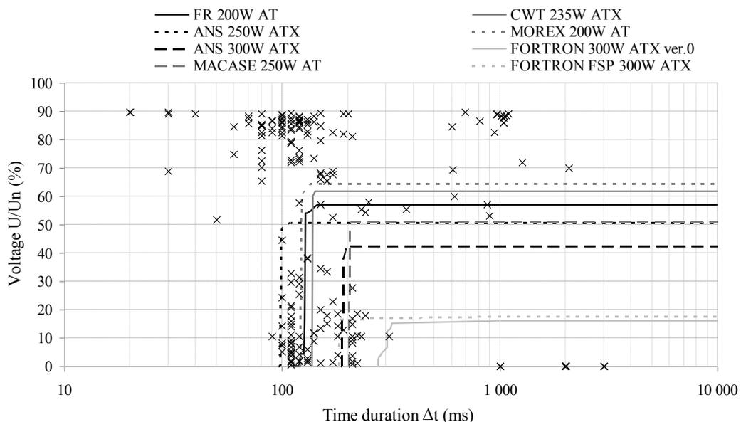
**Figure 3:** Immunity curves of tested computer sources along with mapping of short voltage dips and interruptions
