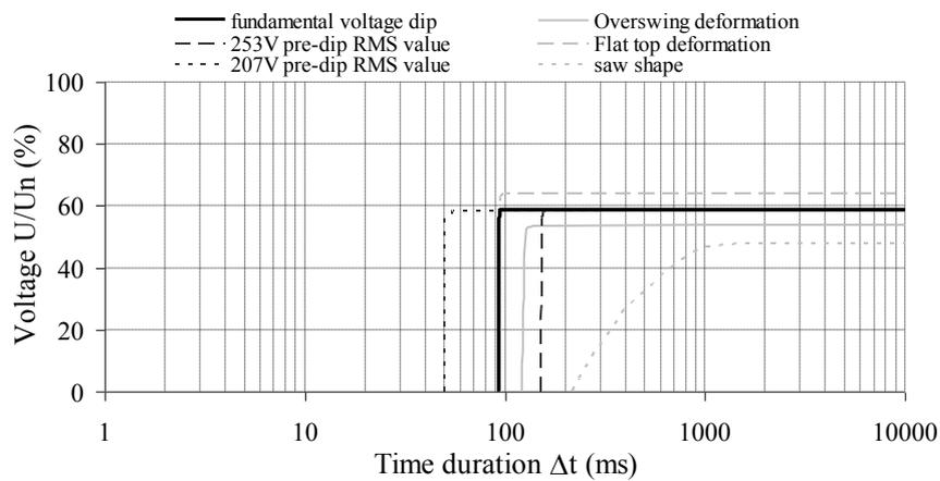
**Figure 2:** Immunity curves of tested computer source CWT 235 ATX for some of chosen dip-parameters modifications [6]. Function criterion: interruption of output supply voltage and computer system was rebooted.
